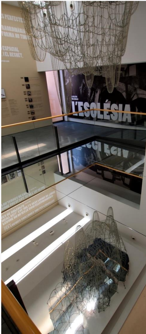
Figure 8. Gaudí's inverted catenary model for the Sagrada Família (c. 1908): weighted cords form structurally optimal parabolic arches when reflected vertically.
