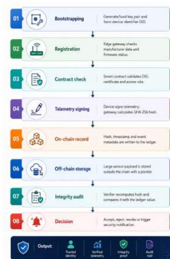
Figure 2. Algorithmic flow of smart-contract-based IoT device authentication.
